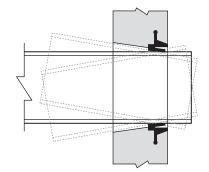
Use a screwdriver to punch out the center of the gasket.
